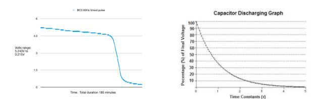
When previously charging the cell to only 1V to 3V I had been capturing only the profile after the cell had begun its steep decline. I had not previously seen the slow ramping down below 5.25V. This demonstrated that for some range of voltages of the blue cells, they were not acting like typical capacitors but possibly were exhibiting indications of being influenced by the actions of magnetic domain alignment, as Steorn had claimed.
