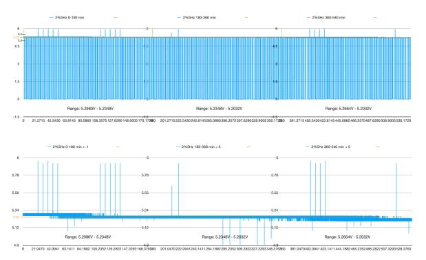
Despite beginning 0.3V higher at the start than the 470 ohm test, this run also moved down to about 5.2V and also showed some large spikes above and below. I'm not sure yet whether those large spikes are artifacts of the recording or not.
