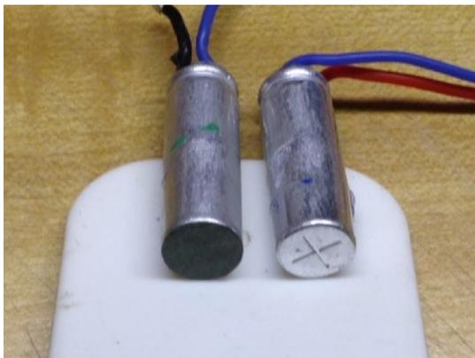
There is a disk between the cells composed of a dense felt-like material, likely conductive.
