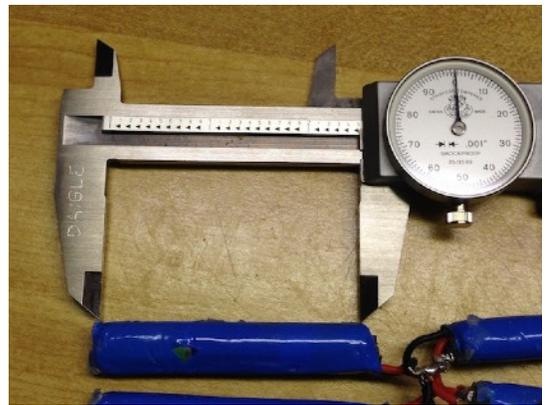
Two of the blue cells with more apparent damage was selected as subjects for testing. Length of the cells is about 2.5".
