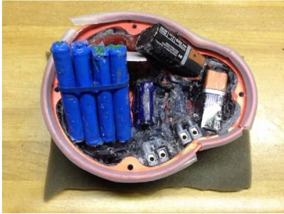
More of the material removed so that now the eight cells can be lifted out, as well as one of the batteries.
