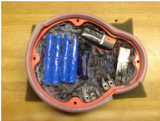
After tape is removed, split polyethylene tubing added to protect the edges of the case from cutting tools. The extent of the matrix material is revealed as well as the positions of the 9v batteries. The matrix is an extremely viscous silicone-like material difficult to remove without cutting or scraping.
