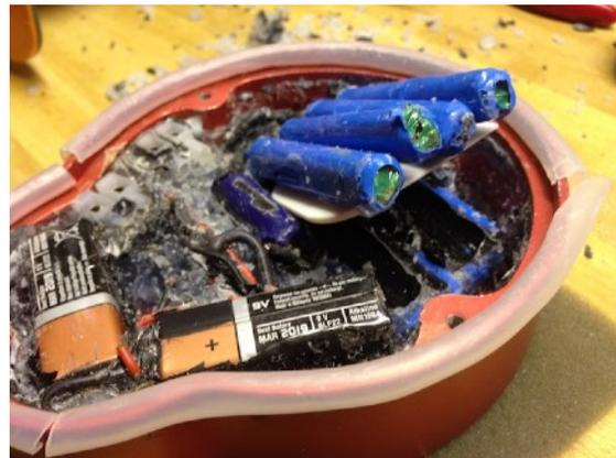
After many hours of scraping and cutting around the blue cells, enough material has been removed to allow the first set of four cells to be pried up.
